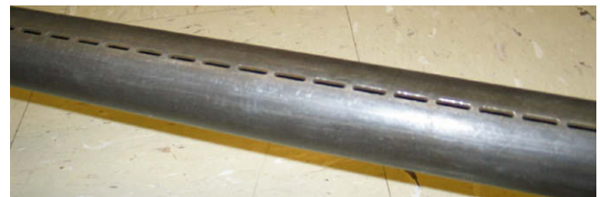
Fig. 2. Photograph of a representative aperture in the array of 39 exit apertures.
